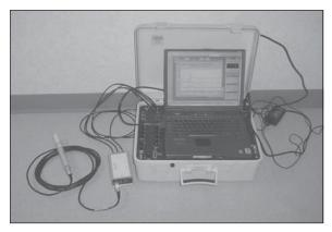
Before installing MRI (magnetic resonance imaging) equipment in a hospital or clinic, engineers on Philips' customer and sales support team visit the site and measure magnetic disturbances and mechanical vibrations that can affect the image. Its engineers must shield and isolate the room from vibrations, or find a more suitable location. Philips has IOtech WavePort/PE8s currently at three locations; New York, Chicago, and Atlanta, with a forth one planned for Irvine, Calif.
